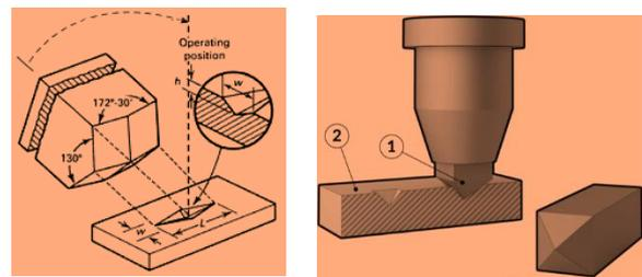
**Figure 5:** Schematic representation of Knoop indenter and Vickers indenter.
