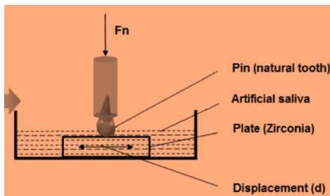
**Figure 7:** Schematic representation Pin on plate test.
