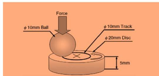
Figure 6: Schematic representation Ball on plate test.
