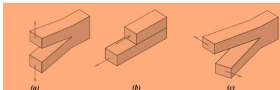
**Figure1:** Schematic diagram showing modes of crack surface displacement (a) mode I, tensile mode (b) mode II sliding mode (c) mode III tearing mode.
