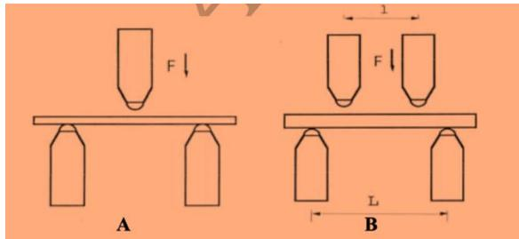
**Figure 4:** Schematic representation of three-point loading test (A) and four-point loading test (B).
