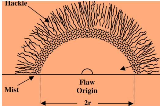
**Figure 2:** Schematic diagram that shows typical features observed on the fracture surface of a brittle ceramic.
